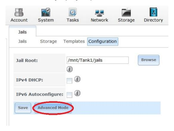
In advanced mode we can now control the IP address range available to the jail/s. This is important because we want the IP address range to be separate and outside the IP address range of the DHCP server in the router. Jails did not work properly for me until I did this.
