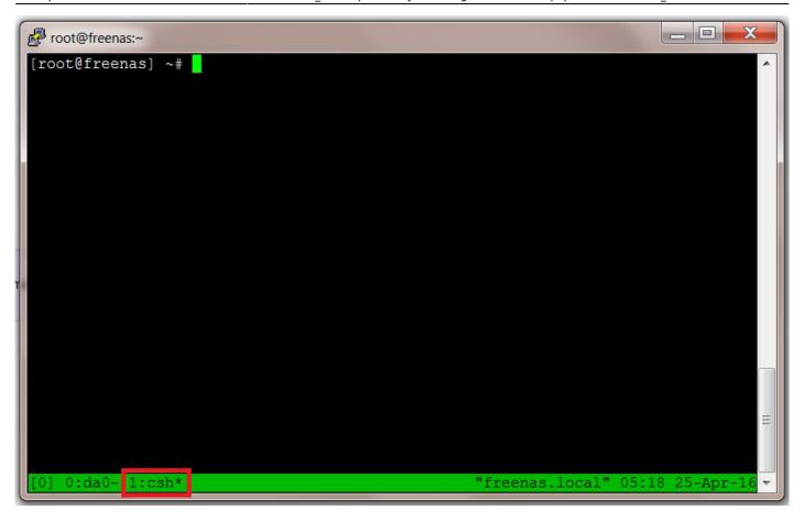
Let us rename this session by pressing the "Ctrl" and "b" keys together, releasing them and then pressing the "," key. Type in the new name and press the "Return/Enter" key (just as we did before, I called this one "da1" after the next drive to be tested).
