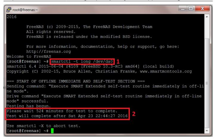
We now need to repeat this process for each drive in the system. We do not need to wait for this drive to complete its test before starting another on a different drive.
